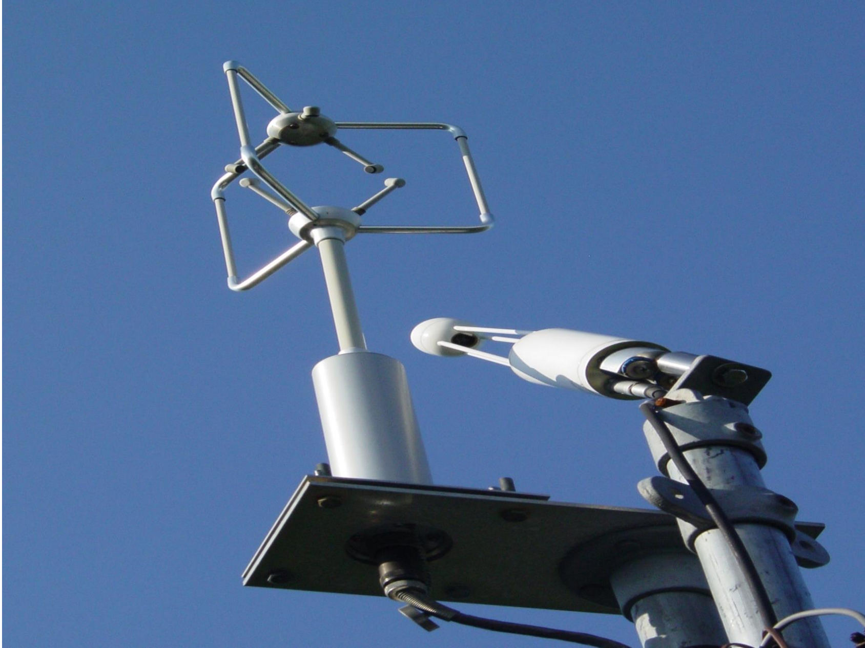
Eddy covariance system consisting of an ultrasonic anemometer and infrared gas analyser (IRGA).
