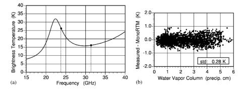
Fig. 2. (a) The microwave spectrum of the atmospheric downwelling radiation at the surface in the vicinity of 22.24 GHz water vapor line for 3 precip. cm of water vapor. The two radiometrics MWR frequencies at 23.8 and 31.4 GHz are indicated by •. (b) The residuals between MWR measurements and model calculations at 31.4 GHz based on the PWV values retrieved at 23.8 GHz as a function of column water vapor (2258 clear sky cases).
