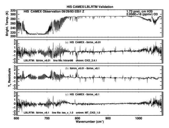
Fig. 1. The top panel is the observed HIS CAMEX spectral radiance provided by the U. of. Wisconsin–Madison. The bottom panels are residual plots of (a) HIS CAMEX–LBLRTM\_v6.01 with HITRAN96 spectral line parameters and CKD 2.4.1 continuum, (b) the difference between the two LBLRTM\_6.01 with HITRAN96 and LBLRTM\_v8.1 with tes\_v\_1.0 spectral line parameters calculations, and (c) HIS CAMEX–LBLRTM\_v8.1 with tes\_v\_1.0 spectral line parameters and MT\_CKD\_1.0 continuum.
