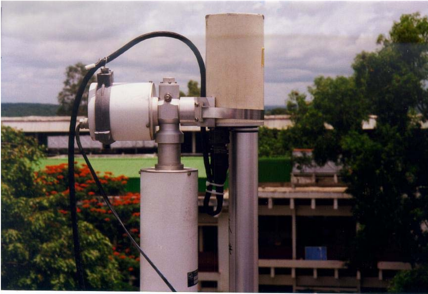
This is how the sun-photometer used by the NASA network looks like. Ilorin, Nigeria
